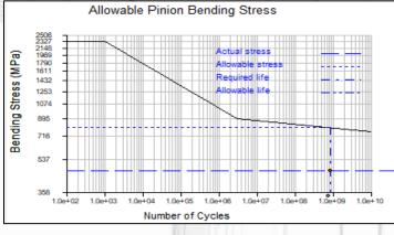
Visual Identification of Safety in Up to 100 Load Cases in Duty Cycle
