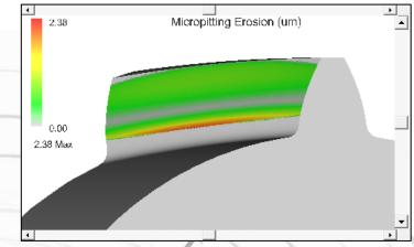
The Wear Due to Progressive Micropitting can be Viewed in 3D at Any Stage
